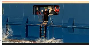
A pilot ladder improperly deployed; not resting against the hull of the ship with no hand rails at the top. Note, also, the steel structure on the hull hindering a clean pilot boat landing.
